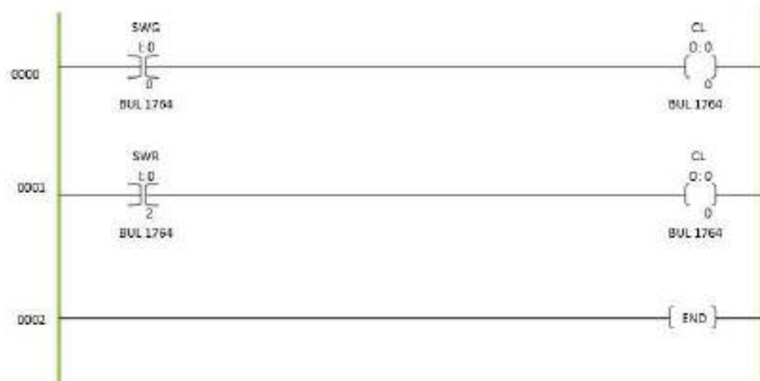
Figure 3.3.6 Program code to actuate a pneumatic cylinder
